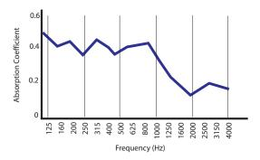
Absorption Coefficients and Noise Reduction Coefficient for the product were measured by an independent, accredited NVLAP facility according to the test methods as defined by ASTM C 423 and ASTM E 795. Random incidence Absorption Coefficients for the product in an E-400 mounting shall be as follows:
