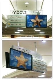
The centerpiece of the customer service sign is its 0.61m x 1.22m (2' x 3') lenticular graphics display, which employs a specially prepared (interlaced) image and a lenticular lens to produce a sequence of images. For instance, (above) a marching bandplays within the star, while (below) fireworks explode. The display is pop-riveted to the clamshell for structural support.
