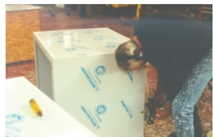
Seams are routed to leave a smooth, clean joint
