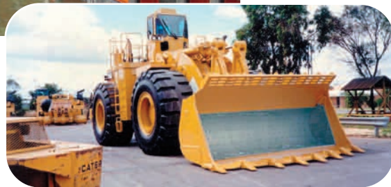
Bucket liners made of Polystone® Matrox™
