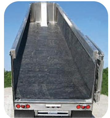
A truck bedliner made of Polystone® M
