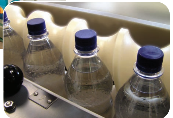
A timing screw machined from Polystone® M-Soft
