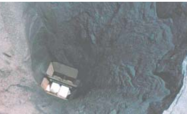
Rathole: The center portion of the bin empties first in the form of a funnel Photo Courtesy of Solids Handling Technologies, Inc.
