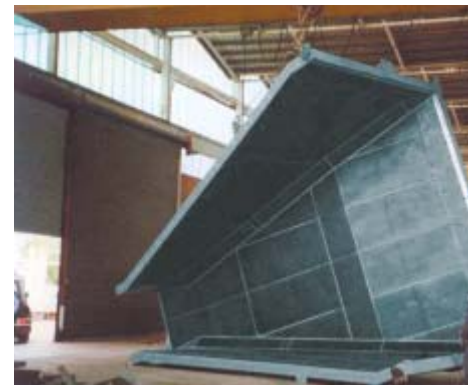
Large chute lined with Polystone® Matrox™
