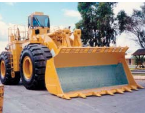
Front-end loader bucket lined to eliminate sticking
