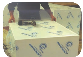
Polystone® sheets are easily cut and welded
