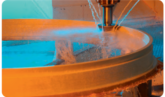
Machining of a Durostone® support ring
