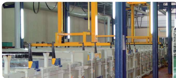
Polystone® P homopolymer grey Galvanic plant for the treatment of aluminum parts
